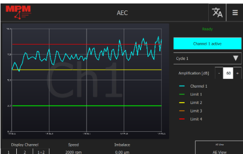
AE acoustic emission sound signal. Limit exceeded
